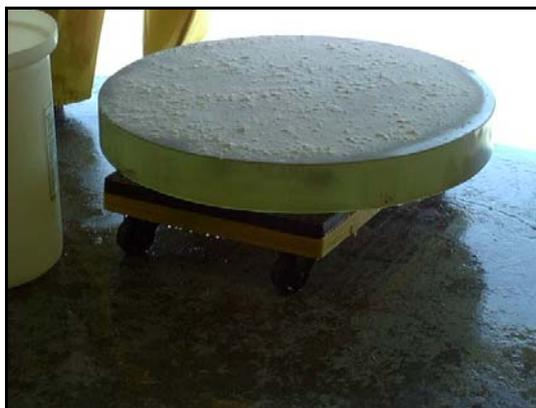
Apply a solution of potassium hydroxide to the surface, then sprinkle on a layer of calcium carbonate.
