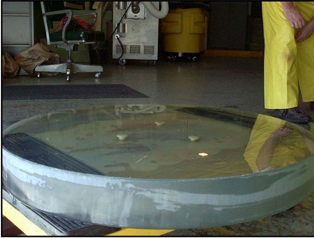
Using Kaydrys, quickly dry surface. The trick is to not allow water droplets to form. Again, use care not to introduce water from sides of glass onto surface.
