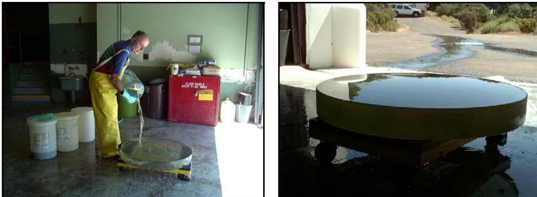
After tap water rinse, thoroughly rinse with distilled water. Quantity used is about 7 gallons. Water will form a nice even layer (no beading, which would indicate some sort of contamination).
