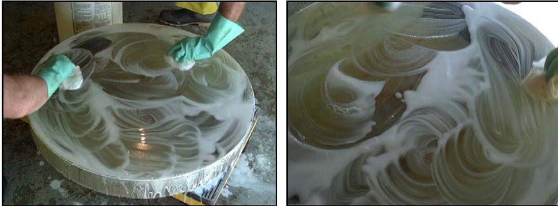
Using the solution of potassium hydroxide, gently rub the calcium carbonate onto the surface, using moderate pressure. It's important to only work the surface; don't bring solution from sides of glass up onto surface, as it may contain remnants of grinding compound. After thorough rubbing, rinse once again with tap water.
